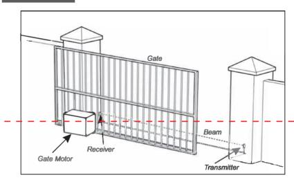
The above drawing shows a standard application of the infrared gate beam sensor used for automatic gate. The transmitter and receiver are mounted at a distance of 30cm above the ground, and they are on the same horizontal line.
