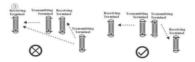
Note 3 : Multiple solar photo-beam shall be installed for long distance, refer picture above for installation instruction
