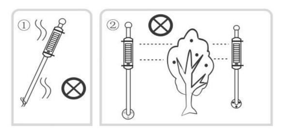
Note 1: Never install at an inclined angle
