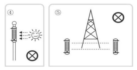
Note 4 : Keep the solar-photobeam holeex-posed to direct sunlight. Note 5 : The high-voltage tower may influence the wireless performance
