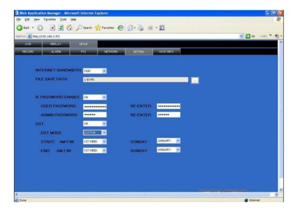
**BANDWIDTH:** Set the amount of bandwidth in kbps (128k, 192k, 256k, 384k, 512k, 1024k) that you want to allocate for traffic that matches internet, this bandwidth not include audio.
