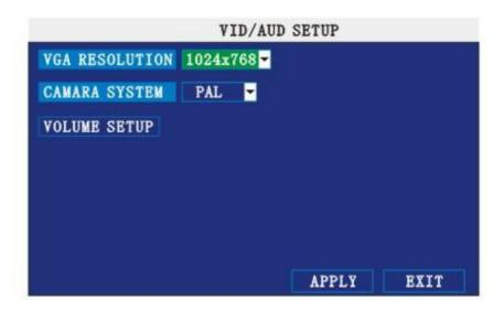
**VGA RESOLUTION:** press [Enter] key to setup the VGA resolution, there are 1024\*768、800\*600 and 600\*480 three options.
