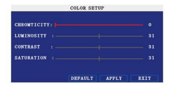
Press [Enter] or directly drag the cursor to set colors,including chroma,brightness, contrast and saturation, press [APPLY] to save the parameters.
