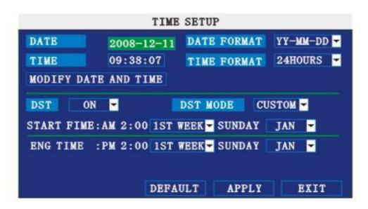
**DATE:** Setup system date via numeric key.
