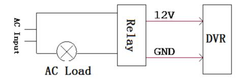
The connection diagram of alarm output as following:
