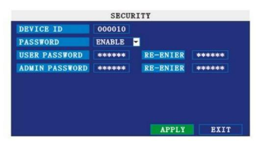
**DEVICE ID:** Press number key to setup the unite ID
