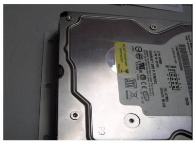
5) Fix the HDD plate on the DVR device and then cover the DVR and screw.
