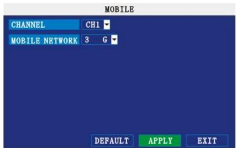
**CHANNEL:** select the channel for mobile view, and press [Enter] to switch different channels.
