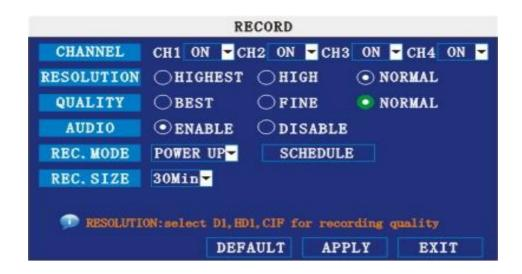
CHANNEL: ON: Means the channel enable for recording.
