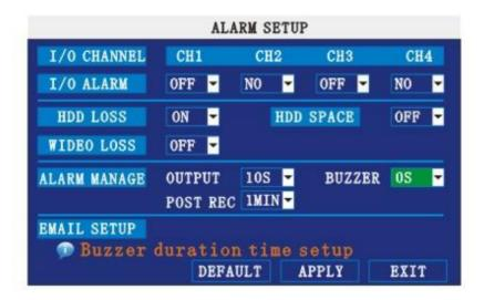
**I/O CHANNEL:** Each channel corresponds an I/O status, that is, when an alarm triggered, it will activate the corresponding channel to start alarm recording.
