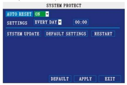
AUTO RESET: When switch is on, you can setup the time for device to restart.
