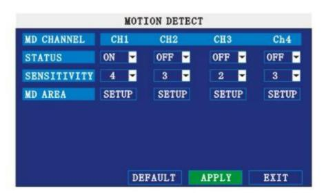
**STATUS:** Each channel has corresponding channel switch, press **[**Enter**]** to turn on or turn off the motion detection for each channel..
