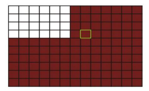
Move the direction key on romote control to make cursor move in the small pane, green frame means the cursor has moved to this pane, press [Enter] to select or cancel motion detection of this small pane, when setup finished, press[exit] to back to MD setup interface, it will save automaticly.
