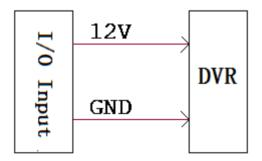
Connection diagram of AC alarm input as following:
